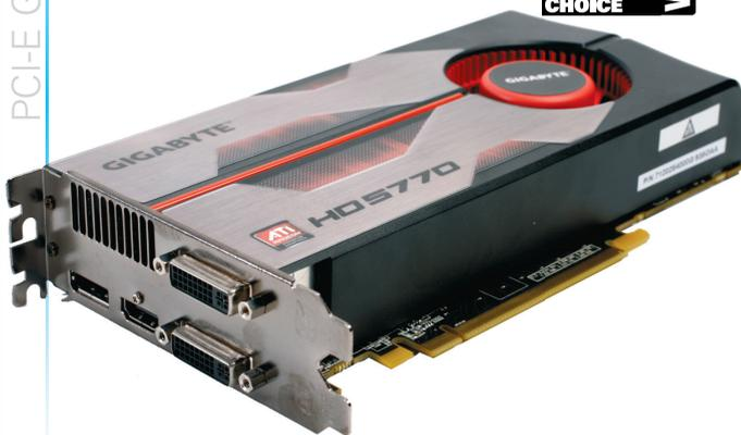
AMD's 5700 series consists of two GPUs – the 5770 and 5750 – both of which target the mid-range market. The 5770 GPU powering Gigabyte's GV-R577D5-1GD-B card is the higher end part of the two models.
